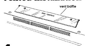
Remove screws from vent baffle on top of range hood. Remove vent baffle.
